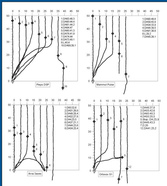
Fig 3. Trajectories of four different 3-antenna beacons in good coupling position. The numbered rhombi indicate the first signal and are discussed in the text. The useful range of the beacons, clockwise from the top left are 30 m, 15 m, 20 m, and 15 m.
