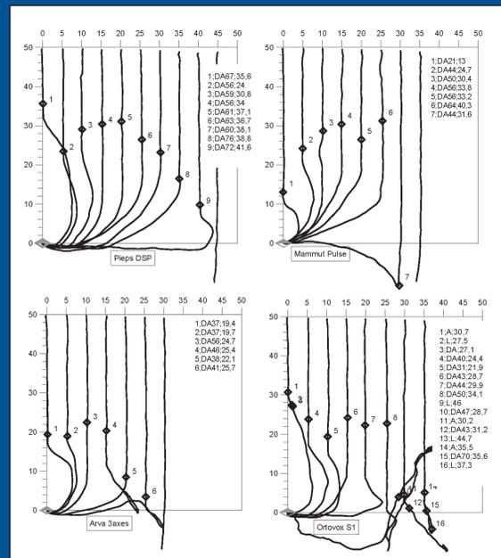
Fig 4. Trajectories of four different 3-antenna beacons in bad coupling position. The numbered rhombi indicate the first signal and are discussed in the text. The useful range of the beacons, clockwise from the top left are 40 m, 30 m, 25 m, and 25 m.
