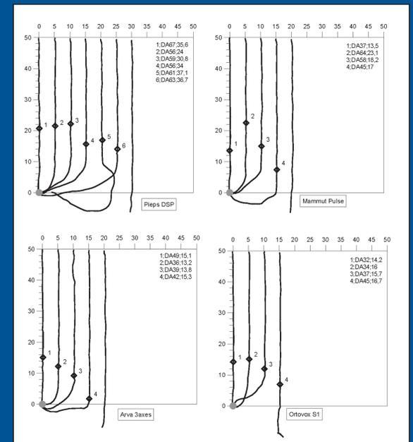
Fig 5. Trajectories of four different 3-antenna beacons with a vertical transmitter antenna. The numbered rhombi indicate the first signal and are discussed in the text. The useful range of the beacons, clockwise from the top left are 25 m, 15 m, 15 m, and 10 m.
